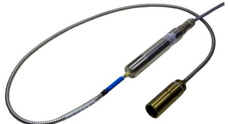
The IGA 320/23-LO is a short wavelength infrared measuring instrument with fiber optics and internal digital signal processing capabilities. This pyrometer is used for measurements of metallic surfaces, graphite and ceramics, etc.
