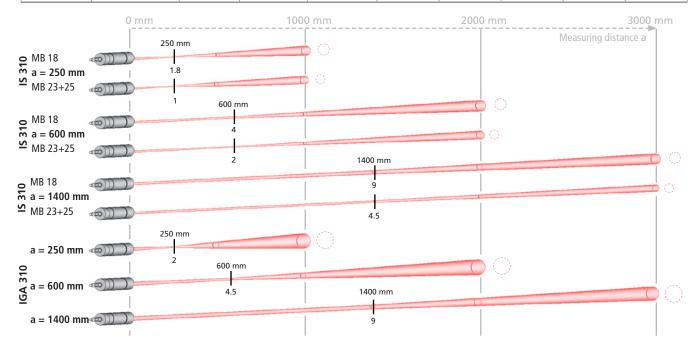
\*) a:M; distance ratio (90% intensity), M: spot size, a: measuring distance, D: aperture (effective lens diameter)
