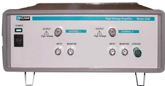
Figure 3 – TEGAM’s Model 2350 Dual-Channel Power Amplifier.
